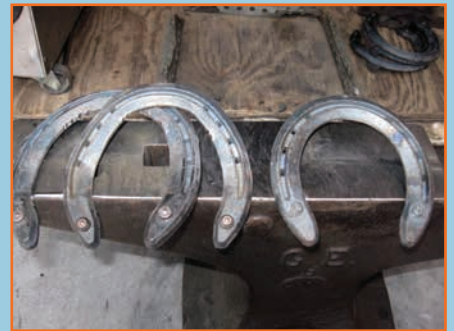
Two shoes with studs on the left, shoe with borium on the right.
